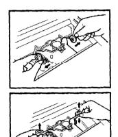
Pass the new tape through the left guide, behind the ribbon guide, and out through the right guide. The rough side of the tape should face the platen.
